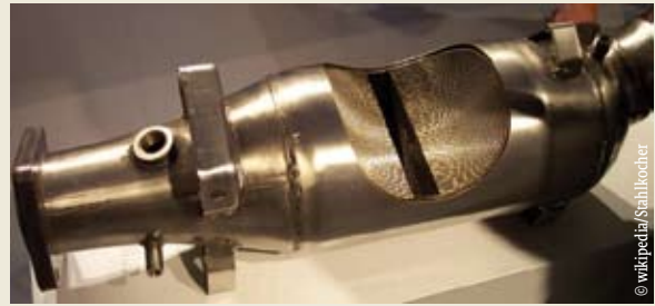
Cross-section of a metal core catalytic converter
